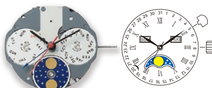
6P80 Height 3.85mm / Date pointer 1 eye (Moon) / 2 Discs (Day/Month) 3 year battery life (SR621SW)
